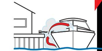
**Blockage of exhaust outlets** can cause carbon monoxide to accumulate in the cabin and cockpit area - even when hatches, windows, portholes, and doors are closed.
